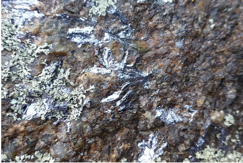
Figure 4 Molybdenite, chalcopyrite, quartz and fluorite vein
